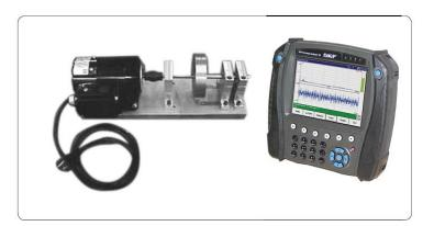
The Rotor Kits simulate the dynamic motion of a rotating machine in a compact, easy to use package. Ideal for class room or laboratory use, the rotor kit may be used to demonstrate vibration phenomena found in large rotating equipment.
